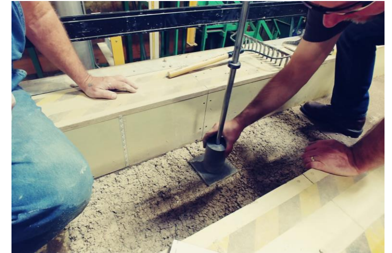
Soil mix compacted in the test box
