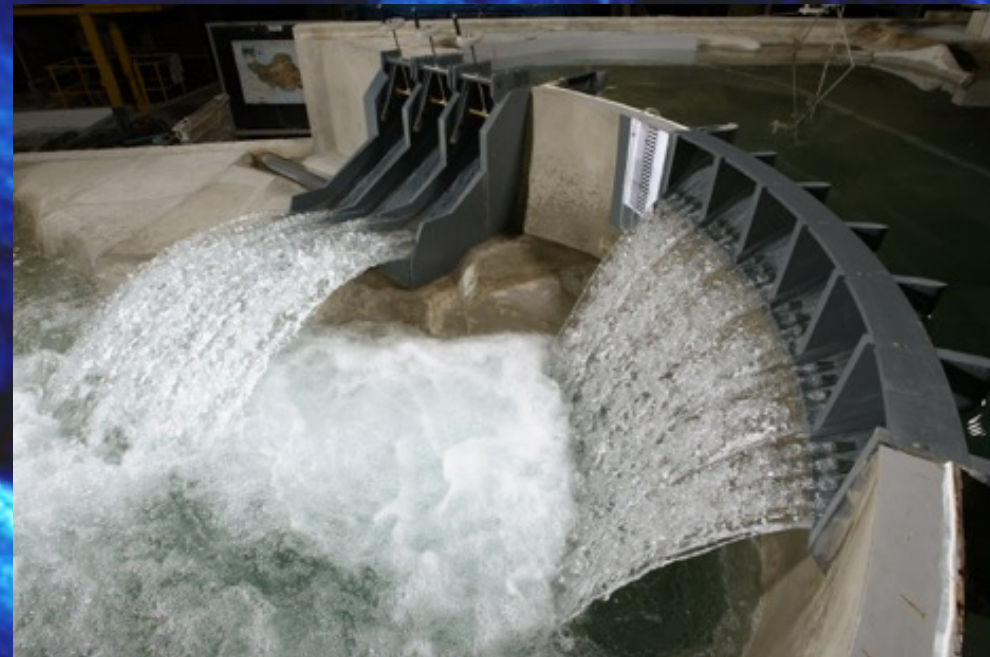
Hydraulic model tests at LCH for Ostour dam in Iran
