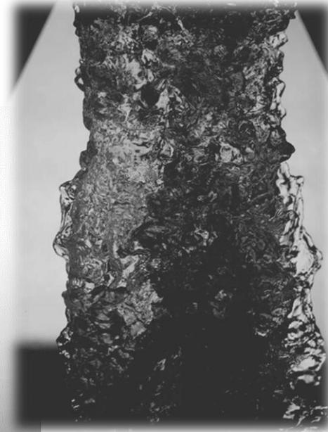
*Jet diameter 135mm, height 1m, flow rate 110 l/s, 7200fps*
