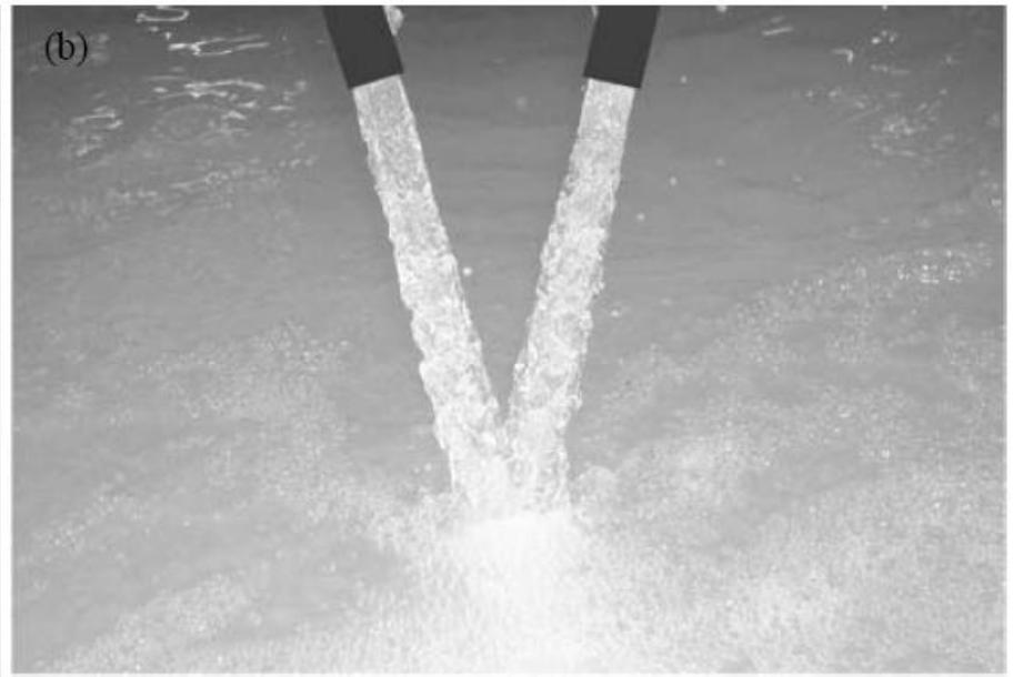
**Figure 4.** Pictures of multiple (a) vertical ( $\alpha_1=30^\circ$  and  $\alpha_2=60^\circ$ ) and (b) symmetric ( $\alpha_c=30^\circ$  and  $\alpha_v=60^\circ$ ) crossing jets
