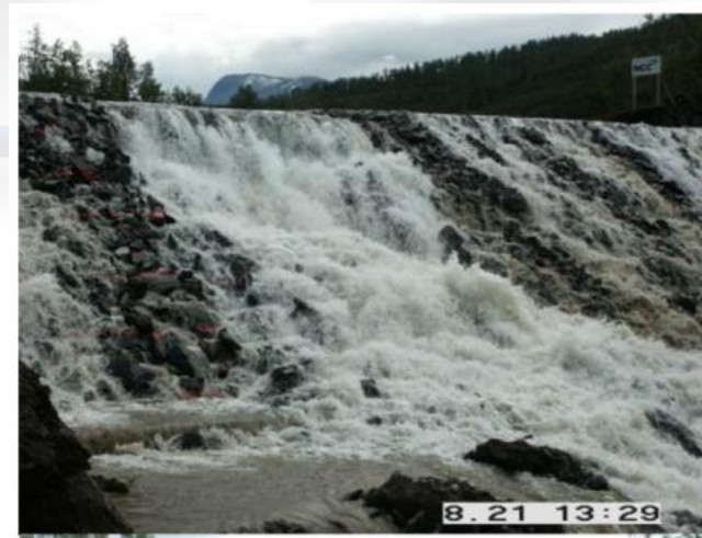
Norway overtopping large scale test
