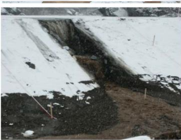
Norway overtopping large scale test
