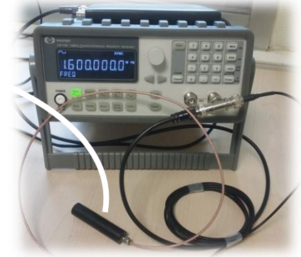
Acoustic sensor for scour depth monitoring
