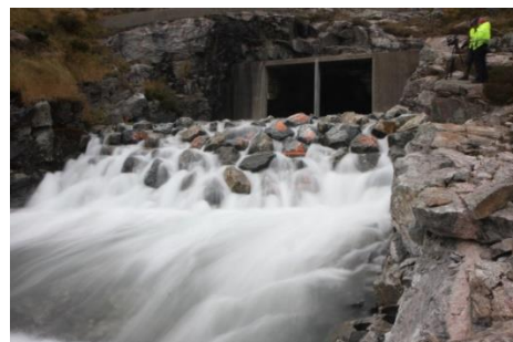
Step 2, Throughflow without overtopping
