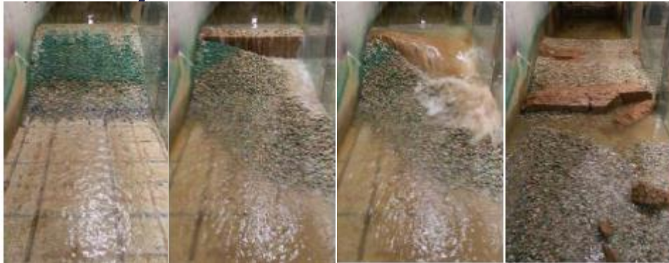
M.A. Toledo, R.M. Alves, R Morán Structural failure of the clay core or the upstream face of rockfill dams in overtopping scenario. 1st International Seminar on Dam Protections against Overtopping and Accidental Leakage (2014)
