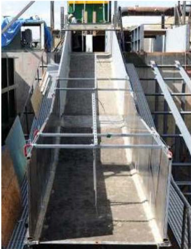
Figure 3-2. Bare clay soil test installation
