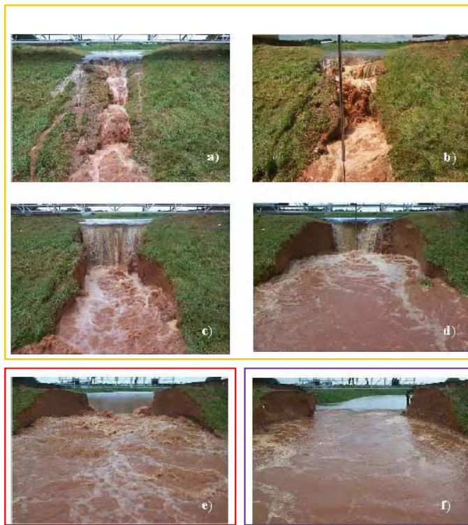
Figure 12. Generalized description of observed erosion processes during ARS overtopping tests: a) rills and cascade of small overfalls during Stage I, b) consolidation of small overfalls during Stage I, c) headcut at downstream crest, transition from Stage I to Stage II, d) headcut at upstream crest, transition from Stage II to Stage III at breach initiation t = t_1 , e) flow through breach during Stage III, and f) transition from Stage III to Stage IV at breach formation t = t_2 .
