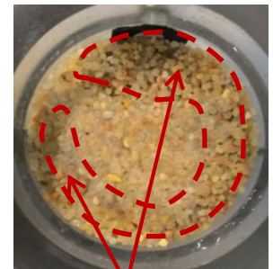
Spread of the erosion zone
