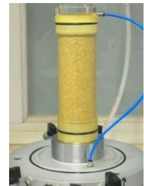
Sample ready for triaxial test
