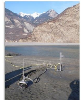
Jet Erosion Test
